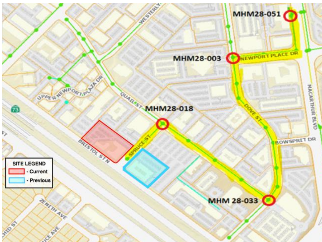
Figure 3. Existing Sewer System at the Project Site
